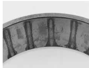
Fig. 189. Staining without pitting.
