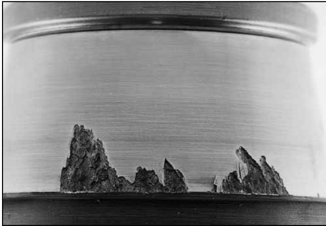
Fig. 171. Geometric stress concentration spalling.
