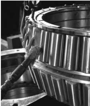
Fig. 245. Lubricating a tapered roller bearing with grease.
