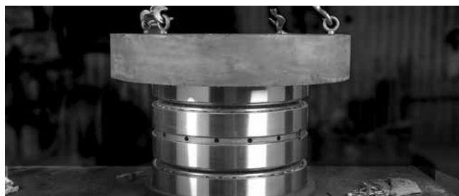
Fig. 265. Applied weight for seating rollers.
