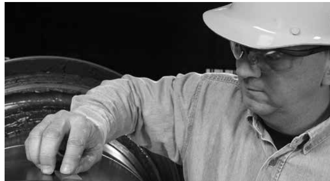
Fig. 240. Restoring minor roll neck damage.
