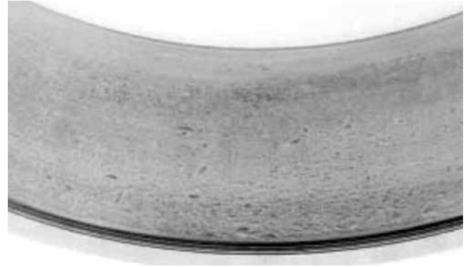
Fig. 160. Bearing damage due to abrasive particles.
