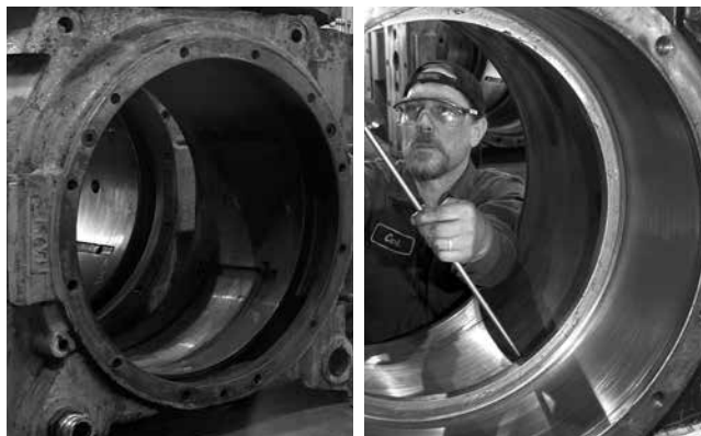
Fig. 278. Chock maintenance before and after photos.
