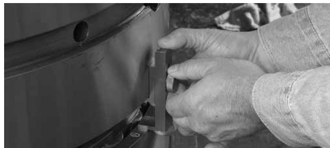
Fig. 268. Measuring B or D gap.
