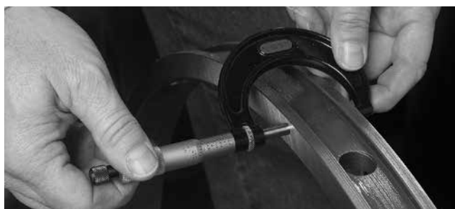
Fig. 269. Measuring spacer width.
