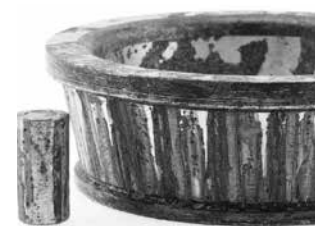
Fig. 192. Damage caused by poor storage conditions.
