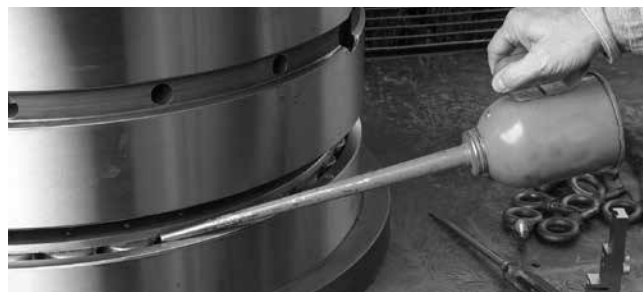
Fig. 267. Applying light oil to rollers and race.
