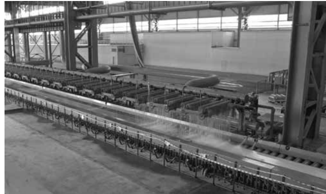
Fig. 110. Hot-strip mill roller tables.
