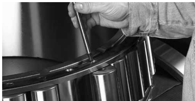
Fig. 232. Removing the threaded pin.
