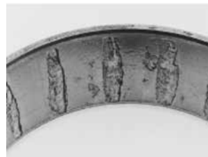
Fig. 191. Deep etching on an outer ring race.
