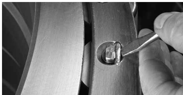
Fig. 231. Removing locking wire from an inspection pin.
